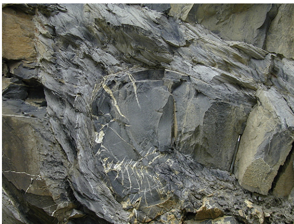
Fig. 9. Hinge zone showing wedge-shaped veins opened towards the outer arc in a competent layer. Tension gashes associated with a shear zone can be seen in the lower part of the picture. South of Isaba. North to the right.
